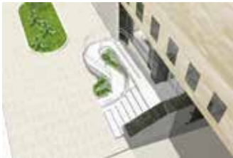
Picture 1.2.1.5. Modifying ramp for a narrow area
