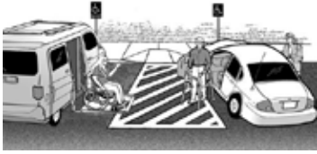
Picture 2.3.1. Sample of importance of side space arrangement of car parking space for persons with disabilities
